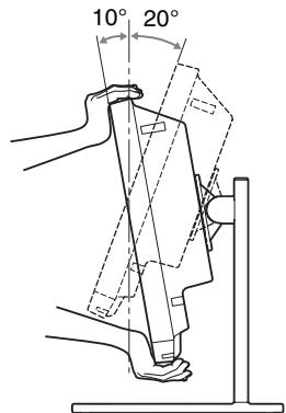
You can adjust the angle by holding the top and bottom of the monitor.
